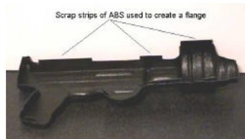
10. The ammo tray after trimming can be installed as-is on the top of the receiver. You may have to notch the back lower edge to get a good fit. The tray should mount flat and parallel on the top of the gun's receiver.
