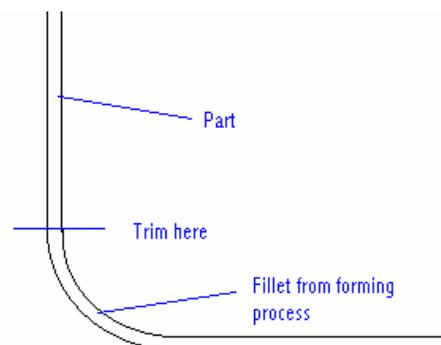
7. Once all the parts are trimmed out, ensure all edges are roughened (not smooth!) to help the glue bond the parts. MEK and a small artist's brush works best (as the MEK causes the ABS to melt and stick together). ABS cement works well. Epoxy or cyanoacrylate (super glue) also works.
